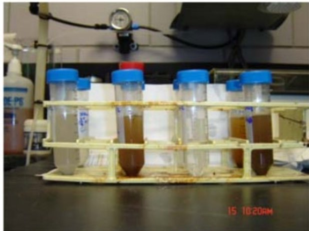
Figure 2. Typical coupon-derived biofilm suspension used for ATP determination.
